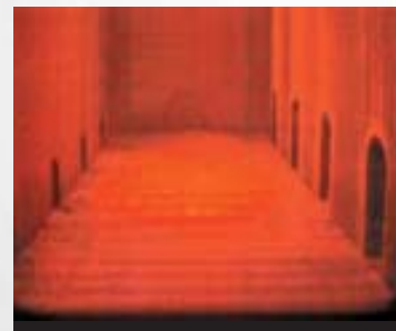
Uniform temperature profile under rider arches with Superflue
