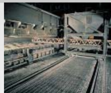
Cold-top electric furnace melting C-Glass and performing at 273 metric tonnes/day (300 US tons/day) at an energy consumption of 775 kWh/metric tonne (703 kWh/US ton)
