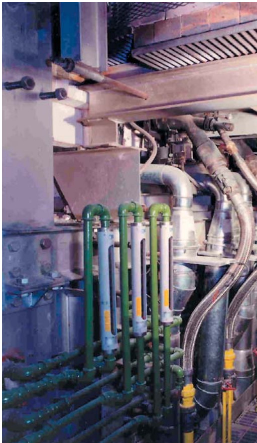
50 sq.m. TECO end-port furnace melting high quality soda-lime container glass
